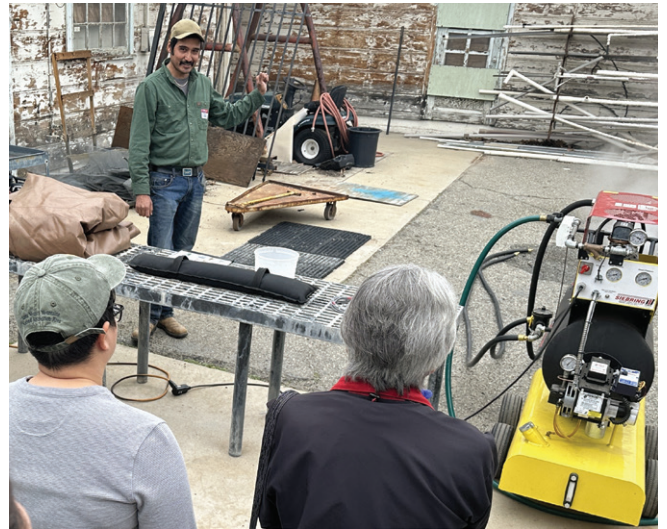
Nursery Manager Ernesto Alvarado demonstrates how to run the soil steamer.
